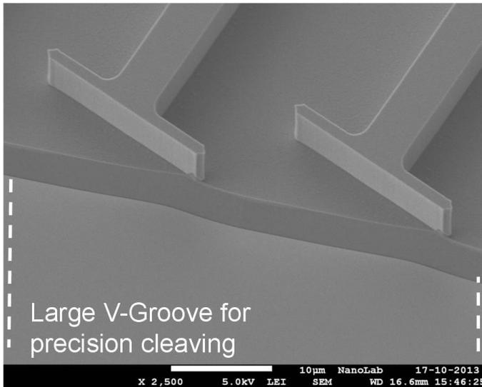
**SEM micrographs of etched facet waveguides produced using an ICP-based etching process illustrate the exemplary characteristics of the resulting structures**
