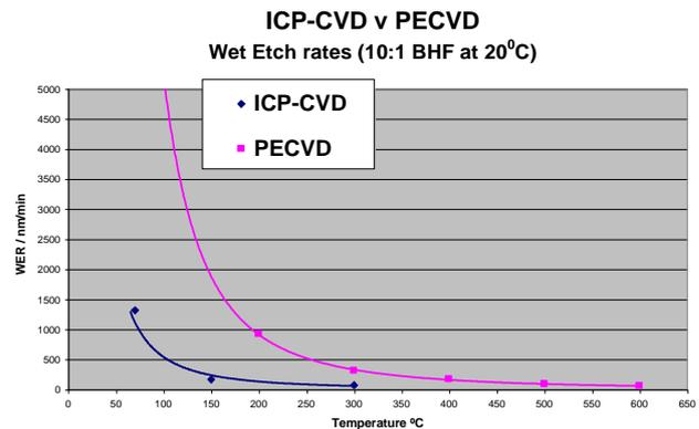
**Figure 8: Wet etch rates highlight the higher quality of SiN<sub>x</sub> films (upper graph), relative to SiO<sub>x</sub> analogues (lower graph), and the ability of ICP-CVD to deliver high quality films at low processing temperatures**
