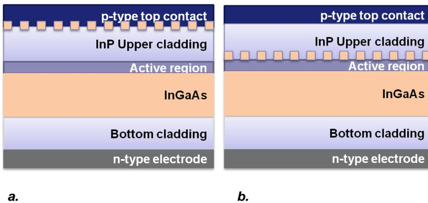
**Figure 1: InP laser structure with a. surface distributed feedback and b. buried distributed feedback**
