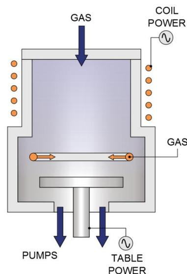
**Figure 3: ICP-CVD enables low temperature**
