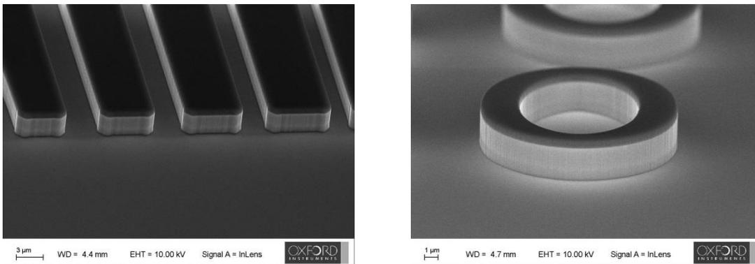
**Figure 10: Using chlorinated process chemistries, ICP-RIE is unrivalled for delivery of the precise profiles and smooth surfaces required for the critical InP Mesa/Ridge etch**
