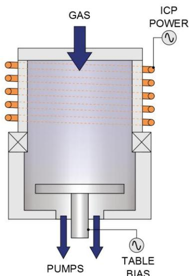
**Figure 5: ICP-RIE delivers high etch rates, at the same time allowing close control of the temperature of the substrate**
