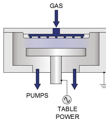
**Figure 4: RIE is a flexible cost-effective option for directional etching**
