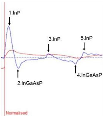
**Figure 7: Laser interferometry can be used for endpoint determination to precisely control etch depth within the manufacturing environment**
