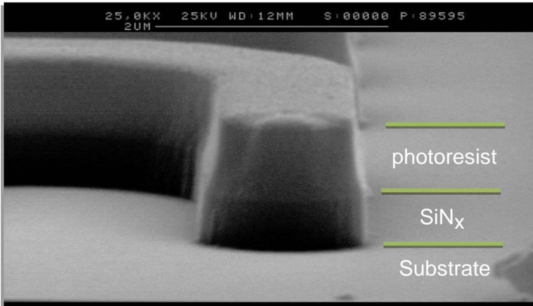
**Figure 9: RIE can be used, along with photoresist, to fabricate a high quality SiN<sub>x</sub> mask for etching of the InP Mesa/Ridge**
