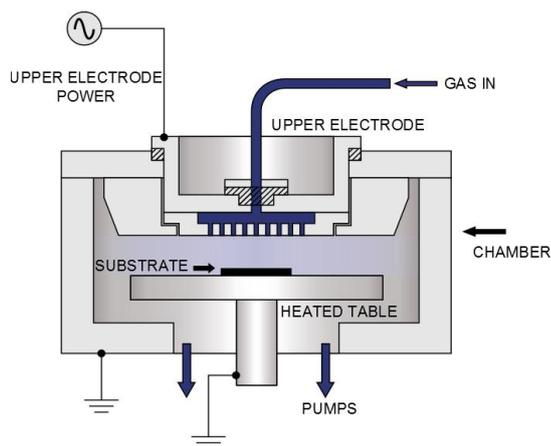
**Figure 2: PECVD enables the deposition of high quality films at relatively low working temperatures**
